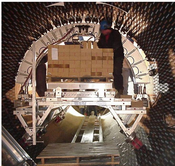
**ST. LAWRENCE CEMENT MULT-O-RING WITH TRAILER & BRICK PALLET CART (FIG 8)**
