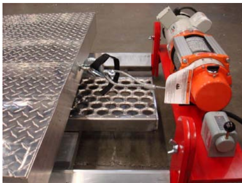
Electric power winch mounted on a platform to ensure cable does not drag sides into end of Port-A-Trac
