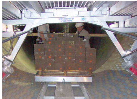
Electric power winch mounted on a platform to ensure cable does not drag sides into end of Port-A-Trac
