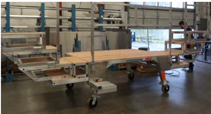
The Bedding Cart is for safe ergonomic refractory installation up to spring line
