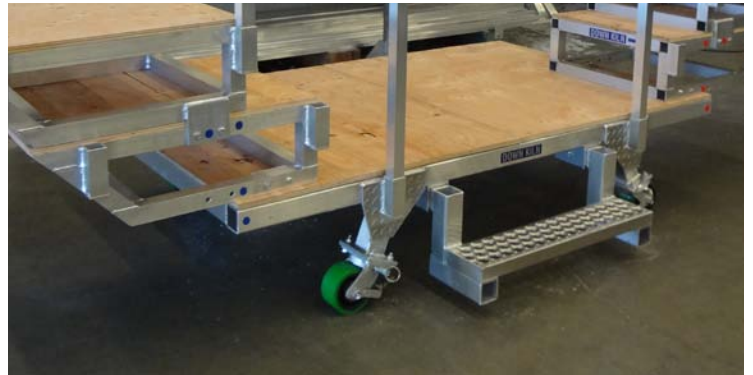
Big castors with kick brake for easy and fast movement of cart, brick, and tools as bedding brick is installed
